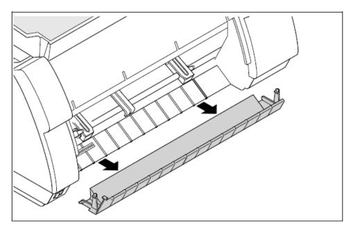
The installation of the optional Front tractor must be performed with the gear of the tractor assembly on the right side. Insert Tractor 2 into the rails on the left and right side walls (as outlined below), in parallel, until the Tractor assembly stops when engaged.
