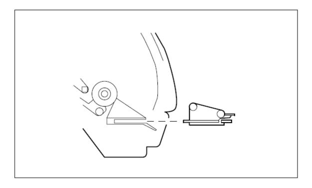
Reinstall the bottom cover and close the front cover.
